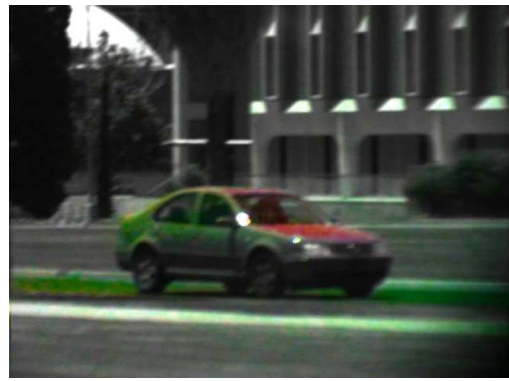
Fig. 10. (Color online) Color fusion image of the vehicle, generated from the spectrally broadband polarization data. Magenta and green represent linearly polarized light with \theta_L \sim -10^\circ and 45^\circ , respectively. Full saturation corresponds to a DOLP of 0.4.
